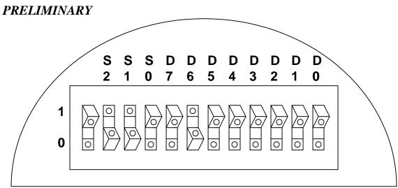
Figure 3. Dip Switches Set to Value [110 01000000] to Reset XRD9827
